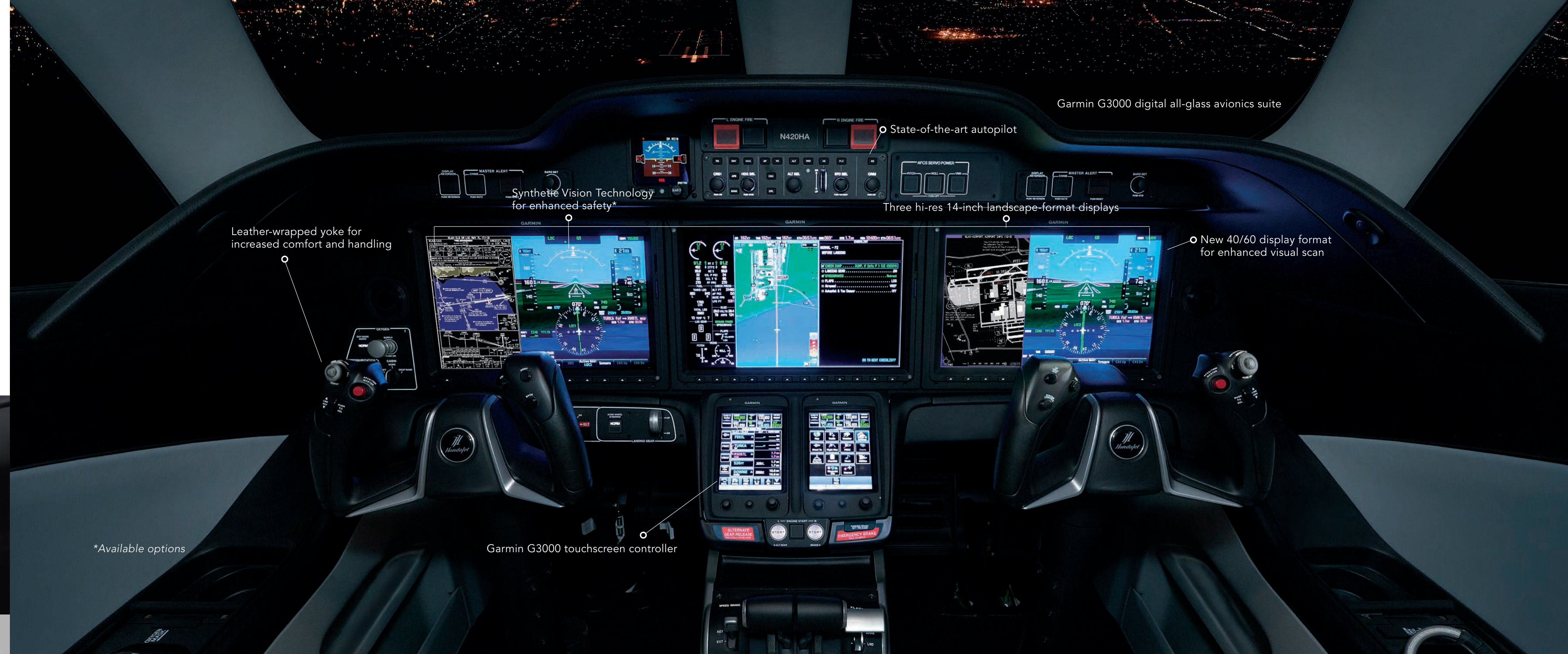
40/60 display format on the Primary Flight Displays enables maximum functional use of display space with easy visual scan for every phase of flight
